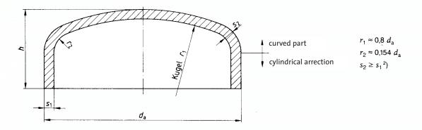
Denotation of a cap according to this norm of a external diameter da = 88.9 mm and a wall thickness s1 = 2.3 mm, at a material of the material group C according to DIN 2609:
