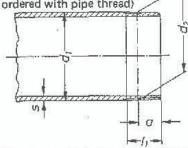
Designation of a seamless medium-weight threaded tube, nominal size 40, galvanized (B), in manufacturing lengths:
